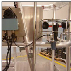
Wind speed control device, with alarm.
